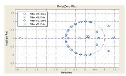
\*\* Filter #1 is the 2(a) design, and Filter #2 is the 2(b) design.
