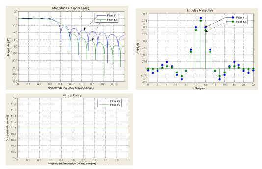
\*\*Filter #1 is the unwindowed design, and Filter #2 is the windowed design.
