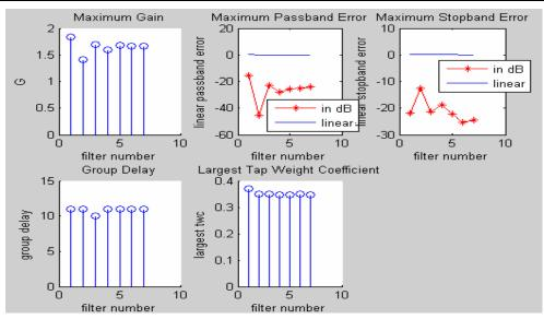
(b) From the figure followed, we can figure out that the group delay is 22-11=11 samples regardless of the input frequency.
