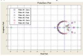
\*\* Filter #1 is the "boxcar" design, and Filter #2 is the Hann design, Filter #3 is the Kaiser design.
