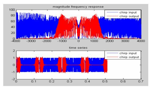
From the figure above, we can see the high-frequency components are gone, which agrees with the predicted filter response, a low-pass filter.
