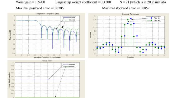
\*\* Filter #1 is the unwindowed design, and Filter #2 is the kaiser design.
