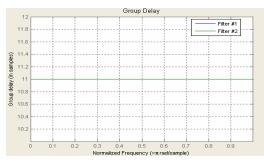
\*\* Filter #1 is the 3(a) design, and Filter #2 is the "boxcar" design.
