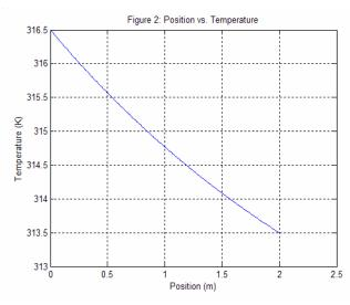
The steady-state quality of this simulation is due to the equal transfer of heat from the bed to the patient and from the patient to the surroundings through convection, conduction, and radiation. Thus, *Equation 3* can be set equal to *Equation 4*, resulting in a fourth-degree equation for the surrounding temperature. Using the "roots" command, MATLAB was used to solve this resulting polynomial, producing one real solution of 296 K. (See Appendix A)
