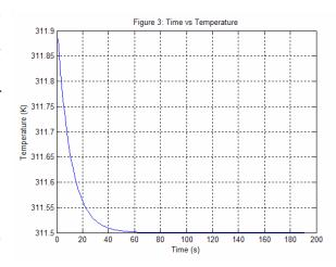
$$Tw(t) = \frac{AK_{p}T_{d} + BT_{p}}{A + AK_{p} + B} + \left[T_{0} - \frac{AK_{p}T_{d} - BT_{p}}{A + AK_{p} + B}\right]e^{-(A + AK_{p} + B)t}$$
