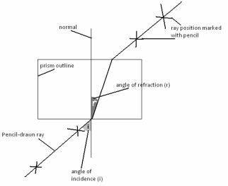
measured with a protractor and recorded (6). This was done another six times for the first set of results. A repeat set of results was then done to increase our chances of getting an accurate result.
