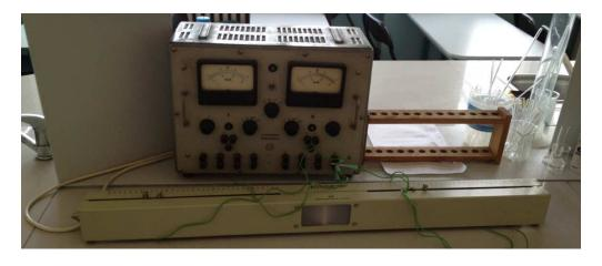
Both surfaces are at the same angle a in respect to their light source. If the illumination on both surfaces is the same and the distance from the source is the same we can derive from the Law of Lambert that:  $I_2 = I_1 (r_2^2 / r_1^2)$ .
