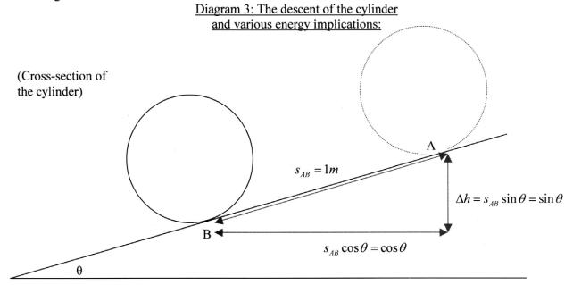
The cylinder has thus lost gravitational potential energy, of an order of:  $E_{\text{potential}} = mg\Delta h \,. \text{ This energy will be transferred in three main forms: in translational kinetic}$
