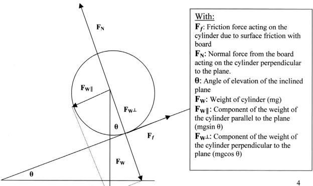
The friction force is the source of the cylinder's rolling motion because it creates a torque about its center of mass, which makes the cylinder roll.
