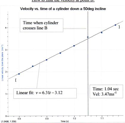
Graph 2: Sample data with 50° incline: How to find the velocity at point B:
