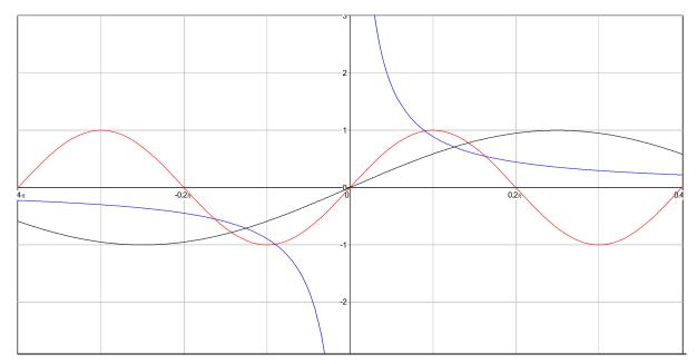
In order to investigate what is the effect of B on the  $y = \sin x$  curve, the graph above has to be compared with the first graph of this assignment, the base graph of  $y = \sin x$ . It can be noticed that B affects the period of the wave. When varying B, it can be noticed that the wave's period is B times as short as the base wave's period. In other words, the inverse of B ( $^{1}/_{B}$ ) is equal to the base wave talking in period terms.
