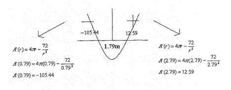
This sign diagram shows us that we have a local minimum and that the value we have for x is indeed the minimum value.
