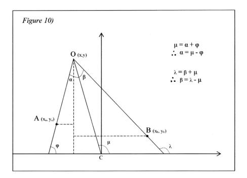
In Figure 10, it is apparent that  $\alpha = \mu - \phi$  and that  $\beta = \lambda - \mu$ . Also, from the
