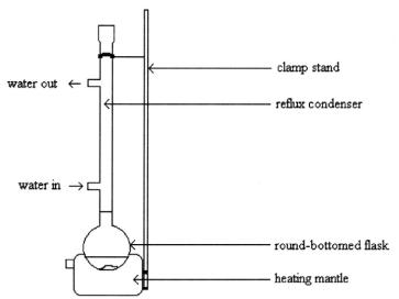
Fig. 11 Esterification apparatus
