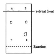
Fig. 5 TLC plate under U-V light.
