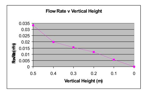
We can clearly see that that Flow rate is proportional to vertical height. In fact the vertical height is one of the biggest factors affecting flow rate. When the vertical height was dropped to 0 m the flow rate was so small that it can be said to be negligible but as vertical height was increased so did the flow rate.
