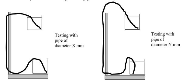
Although the pipes are of exact same length the path the water has to follow is not the same. Since the siphon's performance relies heavily on the pipe's position it is crucial that the pipes follow the exact same path. To do this I will be putting marks on the pipes by using red duck type to indicate certain points on the pipe in relation to the stand. Ex.
