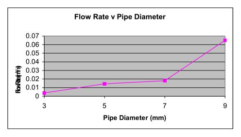
The Flow rate increases as expected with increased pipe diameter. However there is a very large increase in flow rate between a 7 and a 9 mm pipe compared with other increase. Since the increase in pipe size is constant I would have expected the flow rate to increase by the same amount for each pipe increase (a straight line)
