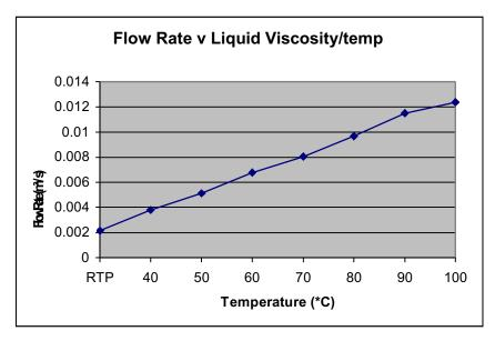
We can clearly see here that a liquid such as olive oil, which undergoes a huge viscosity change with temperature, is directly proportional to the flow rate. For the final test I will be finding the actual viscosity co-efficient as the temperature changes but this is only meant to give us a rough guide to what to expect in the actual test.
