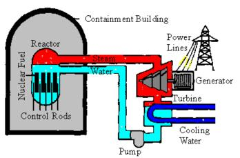
In a BWR, water boils inside the reactor itself, and the steam goes directly to the turbine-generator to produce electricity. Here, too, the steam is condensed and reused.
