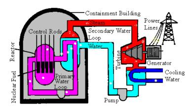
In a PWR, the heat is removed from the reactor by water flowing in a closed pressurized loop. The heat is transferred to a second water loop through a heat exchanger. The second loop is kept at a lower pressure, allowing the water to boil and create steam, which is used to turn the turbine-
