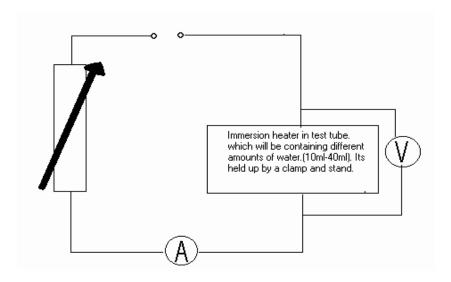
To try and keep this experiment as accurate as possible I am going to try and keep the voltmeter and ammeter to certain values:
