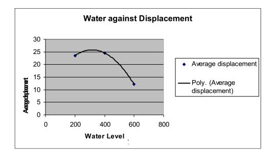
The graph tells me that as the water level increases the displacement seem to have decreased. It seems to me that The Displacement (d) seems to be a function of the water (W). Or  $d = -0.0002W^2 + 0.1063W + 9.1User$  friendly: d = 0.1W + 9 (This is not related to physics but is the relation ship we got when we performed our experiment)
