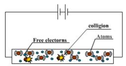
This also can be shown in resistance against temperature graph as in graph 1 where as temperature increases the resistance increase as will, in contrast to this, in a semiconductor, as the temperature increase, the resistance decrease as in graph 2.
