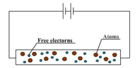
➤ The same metal after the temperature increased, where there are some collegians between the free electrons and the vibrated atoms.
