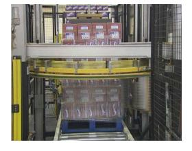
The wrapper is programmed to wrap things up. It shrink wraps the boxes. They are tightly packed up so they don't fall out the lorry. They are very heavy. There is a visual sensor UN the wrapper and a counter to count how many times it goes around.
