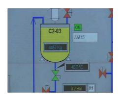
This picture is a chocolate container. I know that this has sensors inside it because we could see the weight and temperature on the computer screen.
