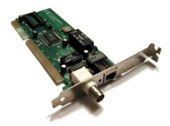
The network card looks like a small circuit board and slots into one of the connectors on the main circuit board (called the motherboard) inside the computer. Network cards have connectors on them from the network cables.
