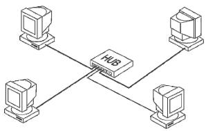
In a star network all the computers are connected separately to the hub or server
