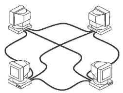
A ring network is a bus network with two ends joined up
