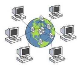
A WAN is a Wide Area Network covering a large geographical area. A wide area network is not confined to one building. The hardware that forms part of the network can spread around the world.
