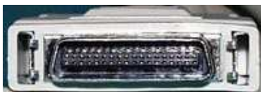
HPCN36 male-This is the new "Type-C" IEEE-1284 Parallel port connector which is used on some new laser printers
