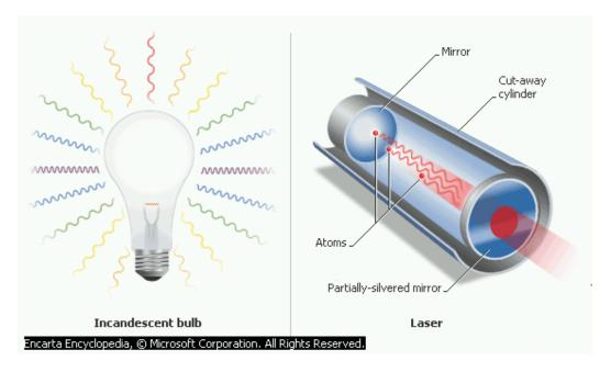
Lasers are generally classified according to the material, called the medium, they use to produce the laser light. Solid-state, gas, liquid, semiconductor, and free electron are all common types of lasers.
