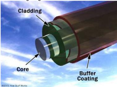
Above shows a diagram of the structure of an optical fibre. (Source: howstuffworks.com)
