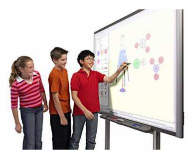
whiteboard sends it back to the computer and the image on the computer is put on the interactive whiteboard through the projector and that is how an interactive whiteboard works. It emits an image from a computer to a screen and then allows you to write on the screen which acts in correspondence with the computer. What's special about the interactive whiteboard is in the name, its interactivity. It ditches old methods of learning to introduce new ways and more involvement.
