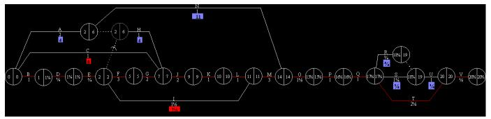
The precedence network would be much easier to read and interpret if it took the form of a cascade activity diagram. I will proceed to introduce cascade activity numbers into the precedence network, making it possible to construct a well-ordered cascade activity diagram.
