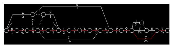
This is only a very simple precedence network; it can be improved if forward and backward passes are included. This will also show the floats for each activity not on the critical path. Only be including more information will I find the shortest time needed to complete the project and maximum times of non-critical activities.
