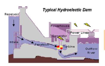
The diagram on the left shows a hydroelectric dam and how it works, as explained earlier.
