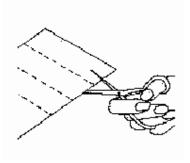
5) Prepare 2-3 strips of chromatography paper. Cut a TLC plate into small stripes e.g. 1.25 x 6.7 cm, so that they fit your tubes. Try not to touch the surface of the plates.
