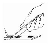
1) I placed 2-4 grass leaves on a slide and then used a second slide to scrape the juice out. I repeated the scarping a few times in order to collect as much of the juice and as concentrated as possible at the end of the slide. A dark "mush" collects at the end. I later removed any larger pieces of debris with a seeker (mounted needle).
