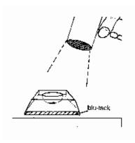
4) Secure the watch glass to bench with Blu Tac and gently dry it with a hair-dryer (2-3min). It should remove all water from the extract.
