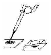
2) I then tilted the slide above the watch glass and added around six drops of propane (acetone) to the green mush and mixed it well. After all that I trickled it all down into a watch glass.
