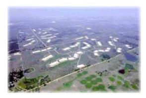
This picture shows rapid infiltration basins (photograph courtesy of Water Conserv II facility, Orlando, Florida) in Orlando, Florida. The water put into these basins recharges the shallow surficial aquifer and is used to irrigate local citrus crop fields.
