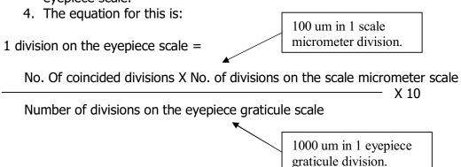
At x100 and x400 magnification the lines on the scale will have a definite thickness. It is important to measure from one side of one scale mark to the same side of the next coinciding mark.
