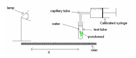
Apparatus: - lamp, ruler, calibrated syringe, capillary tube, test tube, pondweed.
