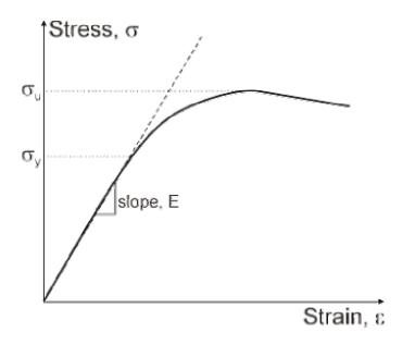
The Young's Modulus is a measure of stiffness and is calculate d using the equation
