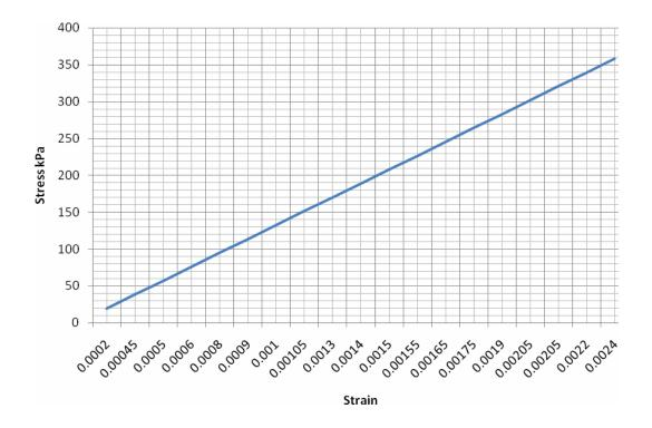
The graph above shows stress plotted against strain. From this graph I can see that stress is directly proportional to strain. The graph however does not show the entire stress strain graph of the material as there is no curve. This suggests that the results were not taken until the material used broke under tension.
