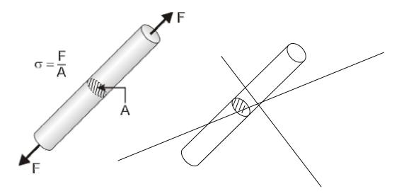
And that strain is extension of the material over the original length  $\varepsilon=\frac{x}{L}$
