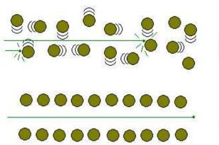
ELECTRONS PASSING THROUGH A HEATED UP MATERIAL
