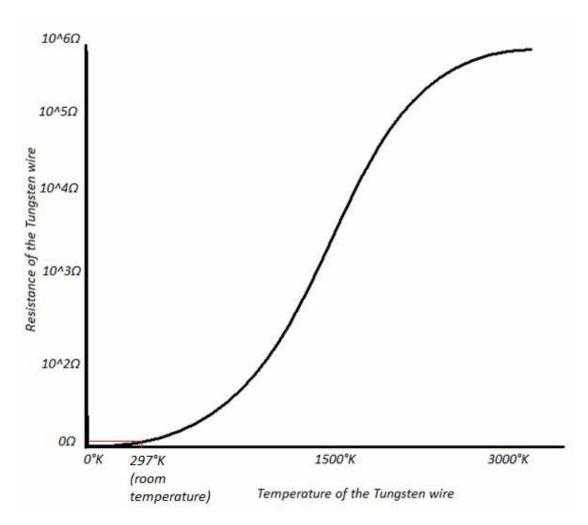
As you can see it's quite a small resistance in comparison to the resistance at higher temperature (like when I turn my bulb on). This graph also demonstrates the amount of resistance there is in the tungsten filament when it heats up.
