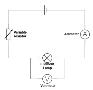
Variable resistor: So I can change the voltage, and thus the resistance in the bulb, so I can draw a table, find the averages, and draw a graph; this would ensure I get as much of an accurate result a possible and minimise any affects that errors wou Id have on my result.
