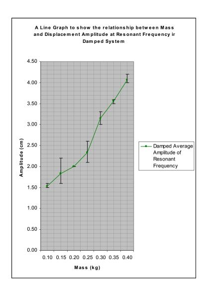
Exactly the same relationships are true as in the undamped system , the values are just lower. The damping effect of water is due to the removal of energy from the system and is caused by friction between the mass and damping fluid. Kinetic energy is lost as heat to the water.
