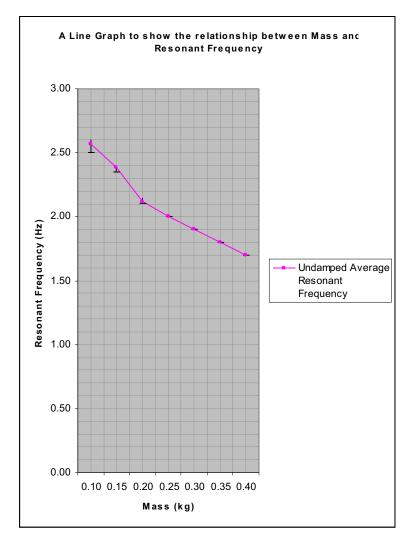
Like the preliminary experiment it was observed that the acceleration of the mass was greatest as it began to move back towards equilibrium and the velocity is greatest as it passes this point. Unlike the preliminary experiment, the frequency does depend upon mass. The graph shows negative correlation between mass and resonant frequency - as the mass was increased, the resonant frequency decreased.
