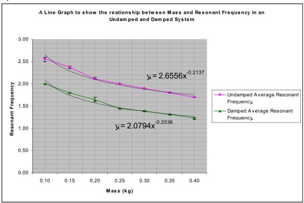
As can be seen in the graph, the resonant frequency is consistently lower in the damped system than in the undamped system.
