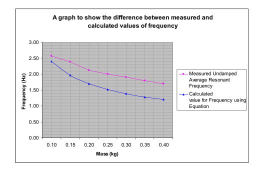
The previous graph shows the discrepancies between observed and expected values, with a difference of around 0.5 Hz. A difference of this nature possibly indicates that the signal generator was producing frequencies approximately 0.5Hz higher than measured.
