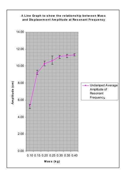
The graph shows that the amplitude at the resonant frequency increases with mass. This is because there is more energy in the oscillating system with greater mass resulting in larger displacement . The amplitude seems to plateau , possibly because increasing amounts of energy are required to extend the spring when stretching it further— in accordance with the square relationship  $E=1/2\ kx^2$ .
