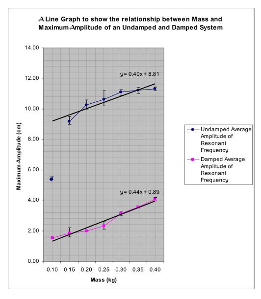
To calculate an <u>approximate</u> percentage change, where the lines of best fit are almost equal in gradient (0.4 and 0.44), the first point was removed. The intercepts differ by 7.92 meaning that, over this range of values, the amplitude is reduced by approximately 8cm by the damping effect of the water. As a percentage change this is:  $(8/8.81) \times 100 = 91\%$ .
