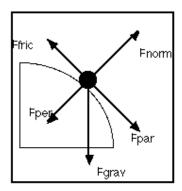
When the object is rolling down the incline, the gravity force has two parts, one is F parallel and the other one is F perpendicular. Fpar = mg sin angle and Fper = mg cos angle. The F perpendicular is balanced with Fnorm, so the ball doesn't move vertically. The frictional force is the force that prevents the car from reaching as high a point which it started.
