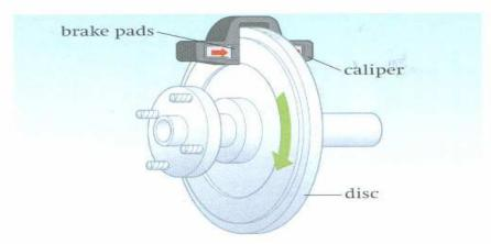
• Figure 7.4 Disc brakes: a metal disc is attached to the axle, next to the wheel. When the brakes are applied, hydraulic pistons push the brake pads against the disc. This provides the necessary torque to slow the car.
