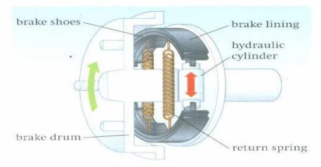
• Figure 7.5 Drum brakes: a metal drum is fixed inside the wheel. When the brakes are applied, hydraulic pistons push the brake shoes against the drum. The linings of the brake shoes are gradually worn away by friction.
