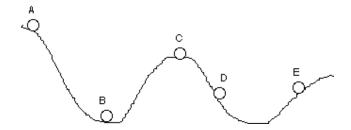
At point A, the car has acceleration and low speed. At B, the car has maximum speed and no acceleration. At C, the car has low speed and no acceleration. At D, the car has the greatest acceleration, because the decline is steeper. At E, the car has the greatest slowing. (See the graph of acceleration and velocity)
