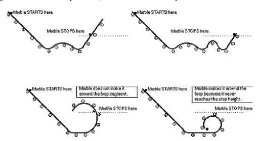
(2) The ball begins to roll down due to the force of gravity. It stops when all the energy gravity gave the ball is used up. The marble accelerates only while a force acts on it *in its direction of motion*.
