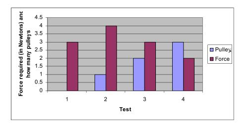
A surprising result has been achieved. The trend is very unusual. I have seen that the more the pulley is added the less force is required. But through observation i can see that without a pulley at all is better that has 1 pulley or 3 pulleys.
