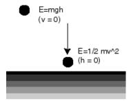
So the kinetic energy of the ball bearing on impact is equal to its potential energy before it is released,  $\mathbf{E} = \mathbf{mgh}$ . Here  $\mathbf{m}$  is the mass of the ball bearing (in kg),  $\mathbf{g}$  is the gravitational acceleration = 9.81 m/s<sup>2</sup>, and  $\mathbf{h}$  is the height of the ball bearing above the sand (in meters). If we drop the ball bearing from different heights, we get different values of energy on impact and different crater diameters.
