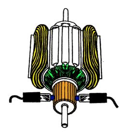
A simple DC electric motor. When the coil is powered, a magnetic field is generated around the armature. The left side of the armature is pushed away from the left magnet and drawn toward the right, causing rotation.
