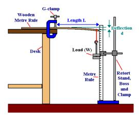
The meaning of deflection is the movement of a structure or a part of a structure when it is bearing a load.
