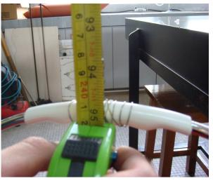
• Use a measuring tape to measure the length of the wire after holding it with a water
