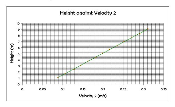
From this graph I can see that it now forms a straight line graph. The gradient is 35.88 and the y intercept is 2.0657. This means that the friction involved is negligible and the ramp acts essentially as a smooth plane.
