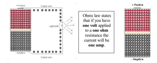
Knowing that, it is possible to calculate the voltage, resistance and current in a circuit if you know 2 of the values using the equations V=IxR, R=V/I and I=V/R
