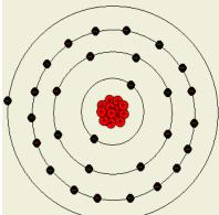
The copper atom has 29 protons in its nucleus with 29 electrons orbiting the nucleus. The electrons are arranged in orbits called shells.
