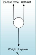
During the course of this investigation I study the effect of temperature on upward viscous force. Since I am using the same ball for all calculations, the weight of the sphere remains unchanged. However the upthrust will have to be calculated at
