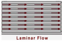
constant. Uniform viscosity throughout the liquid results in layers of flow, at different velocities in relation to one another. Therefore for this kind of experiment it is important that we use liquids with laminar flow (e.g. glycerol).
