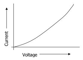
If my line of best fit on my graph is flat, the resistance through the electrolysis cell is high, if the line is steep, the resistance is low.
