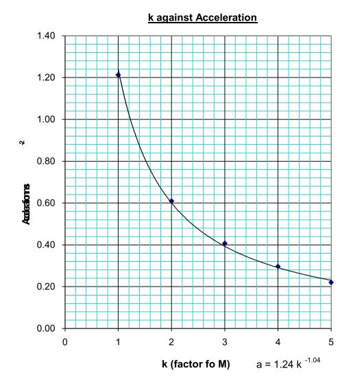
The Graph show that  $\bf a$  is approximately equals to 1.24  $k^{-1}$ . The Acceleration is inversely proportional to k and as k doubles, the acceleration halves.
