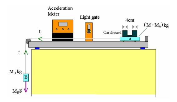
Let M = the mass of the trolley (A),  $M_A =$  Mass added onto the trolley
