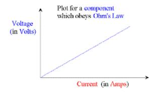
In reality, an increase in current through a component will change its temperature (the temperature usually goes up), and so Ohm's Law is only a generalisation but it works quite well for many components.
