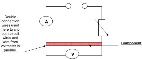
The voltmeter must be placed in **parallel** around the **component** (in this case the wire attached to the ruler). The component, ammeter and the variable resistor are all in **series** and can be placed anywhere in the circuit.
