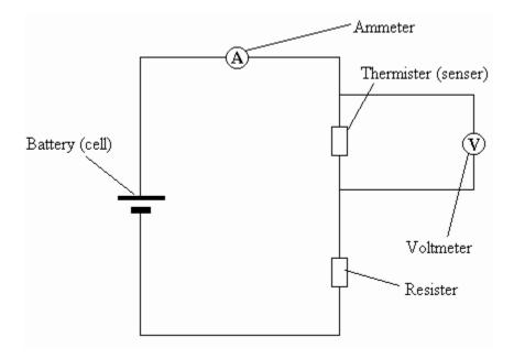
As you can see I have kept the circuit linear to ensure that it is as simple as possible. Two parallel wires will be ran off either side of the sensor in the circuit so that the voltage can be measured, and the current will be measured after leaving the cell.
