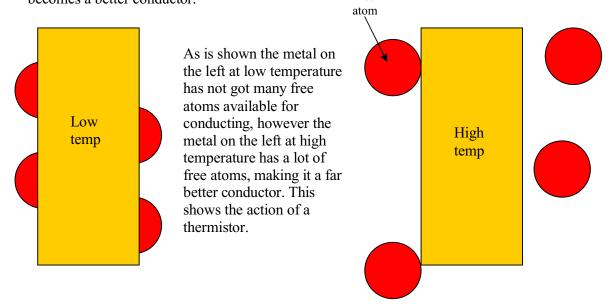
Materials that react like this are called semiconductors. Carbon, silicon are two materials whose resistance decreases as they get hotter. Thermistors can be used for the following functions:
