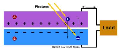
Photovoltaic cells have a positive and a negative layer. The positive layer is made from boron and goes underneath the silicon layer. The process of adding impurities on purpose is called doping, and when doped with boron it becomes P-type silicon. When mixed into the silicon lattice, the Boron forms "holes" in the lattice where a silicon electron has nothing to bond to. Holes can conduct current allowing it to flow through the silicon.
