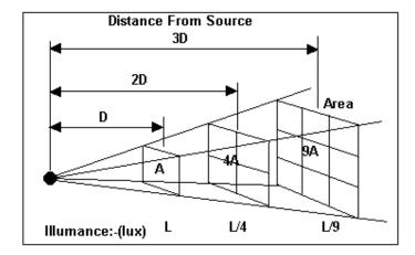
As you can see here, if A is the area of the PV Cell then all the photons travelling in that direction will hit the cell. If it is twice as far away, it will have one fourth of the photons travelling in that direction and if it is three times as far, it will have one ninth of the photons travelling in that direction. This would produce the exponential curve that should be observed by my results.
