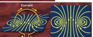
This is the magnetic field around a single loop of wire; there are more field lines a single loop than in a straight piece of wire. If the loop were to be repeated several times it would make the electromagnet much stronger.
