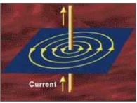
This is the magnetic field around a piece of wire, compared to a magnetic field on a loop or solenoid it is weak. Turning coils around and passing a current through them will make a much stronger electromagnet.
