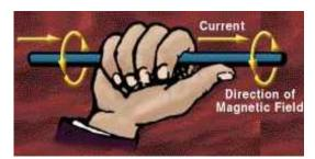
The right hand rule states that if you make a fist, when you point your right hand thumb in the direction of the electric flow, the rest of your fingers curl in the direction of the magnetic field. The direction of the flow of current always goes from the positive end to the negative end.
