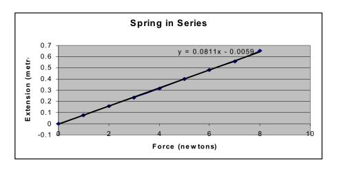
The graph that has been plotted (spring stiffness against load) shows that the stiffness of the spring halves when there is single spring but when two are put in series then the stiffness is doubled. It can be seen clearly that the gradient of single spring is almost half of spring in series.
