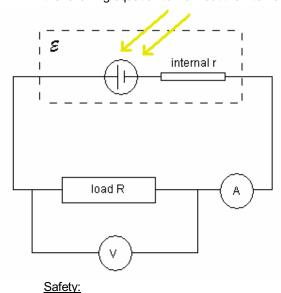
This corresponds to the equation y = mx + C. When V is plotted against I and the corresponding equations y = mx + C and V = -rI + t, then gradient m = -r and C = t The equipment used is not inherently dangerous but care should be taken not to over heat the circuit. The work area should be clear.
