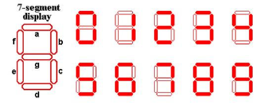
This is what will display the numbers. Has 7 LED sections, available in many colours (most commonly red). I will be using a common cathode display. ▲s a common anode will not work with the 4511 decoder. Common cathode means all the 0ve connections of the LED's are joined, there for having one negative connection for all the LED's. Different LED's are lit to display different numbers. The diagram above shows this.
