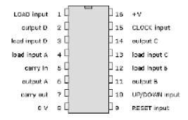
The 4510 BCD (Binary Decimal Counter) counter. Usually has 4 outputs ♠, B, C and D. ♠ being the least significant bit.
