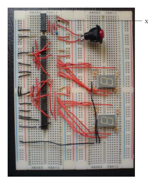
In this diagram I am using a slow pulse system to check the counting system. For the final testing and use I will replace resister X with a series of resistors, with a total resistance of  $14.2k\Omega$ . To get this resistance, I will use the following resistors (from the E24 series) in series.
