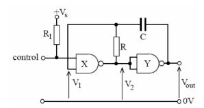
While the circuit is disconnected. There is no charge in the capacitors. When initially switched on. Unbalances in the 2 NAND gates make sure that one output goes high (logic 1).
