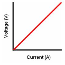
The current and voltage would rise proportionally resulting in a straight line. If you double the voltage, the current will also double.
