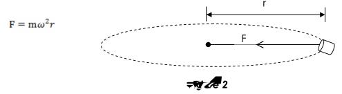
where  $\omega$  is the angular velocity of the circular motion. The force is provided by the tension of the string and it must be directed towards the centre of the circular path.
